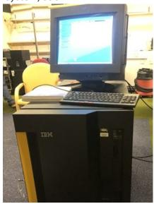
Our recently acquired System/390 including the integrated Support Console which runs a tailored version of OS/2 has been successfully powered up. We now need to work out how to get the actual S/390 to do something useful.
